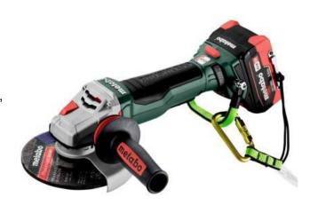
The WPB 18 LTX15-150 Quick with DS grinder has a powerful and fully encapsulated 10,000 RPM, 1100 watt/11-amp equivalent brushless motor for high performance and low maintenance. The grinder also comes with features like Metabo's M-Quick tool free wheel change system, mechanical safety clutch, safety brake, soft start, non-locking paddle switch and overload protection for longer motor service life.
