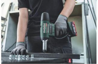
pulling force of 1,500 N or 337 feet per lb. This one-handed rivet gun is extremely fast, lightweight, and well balanced for maximized ergonomics. It also includes safety features, such as a hand protection guard and balancing loop.
